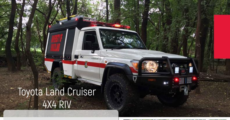
TOYOTA LAND CRUISER 4X4 DIESEL OR PETROL SEATING FOR DRIVER PLUS CREW OF ONE 350 LITRE WATER AND 25 LITRE FOAM ULTRA HIGH PRESSURE FIRE FIGHTING UNIT 42 L/MIN @ 100 BAR FULL WIDTH STORAGE LOCKERS WITH SLIDE **OUT TRAYS** TNT HYDRAULIC RESCUE TOOLS **UPGRADED SUSPENSION** REPLACEMENT BUMPER WITH WINCH RIGID INDUSTRIES LED SCENE LIGHTS WITH LIFETIME WARRANTY DUO SAFETY A FRAME LADDER ALL TERRAIN MUD TYRES 2 x SCBA SETS COMPLETE RIGID INDUSTRIES LED SPOTLIGHTS 7500 **LUMENS EACH**
